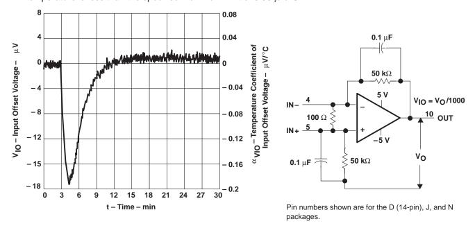
Figure 36. Effects of Package-Induced Thermal EMF
